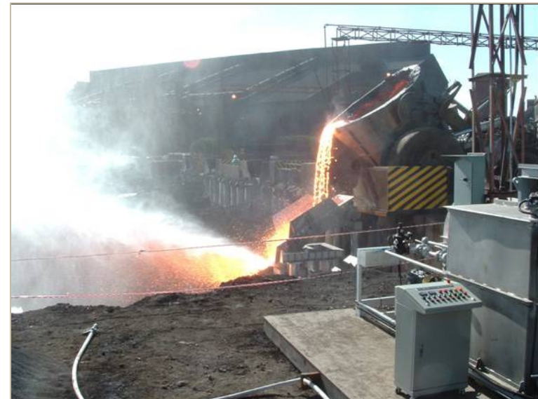
Ecomaister air granulation Producing PS balls (for shotblasting firstly)
